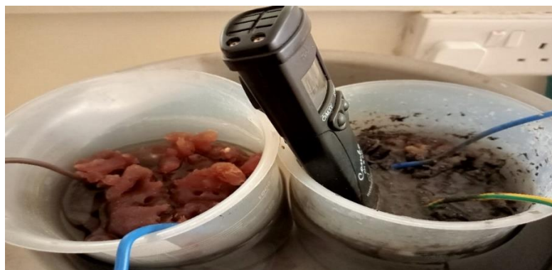
Figure 4: MFC with ash and control setup without ash
