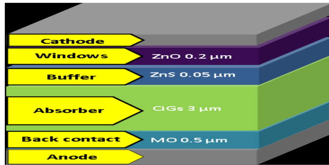
Figure 1. Structure of CIGS solar cell.
