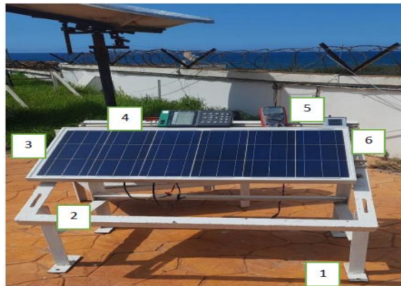
Figure 2. External test bench. 1) mechanical structure with a 36° inclined plane, 2) grouping frame, 3) polycrystalline solar panel, 4) Prova200A solar simulator, 5) Multimeter (LINI-T, UT71E), 6) Reference cell (Si-V1.5TC-BATT).
