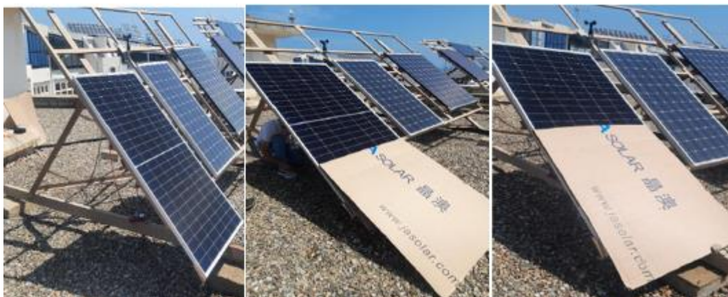
Figure 10. Outdoor test bench the effect of partial shading on the PV module (0%, 25% and 50%).
