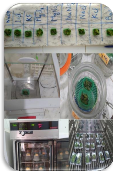
Figure 2. System for the preparation of sorption isotherms.
