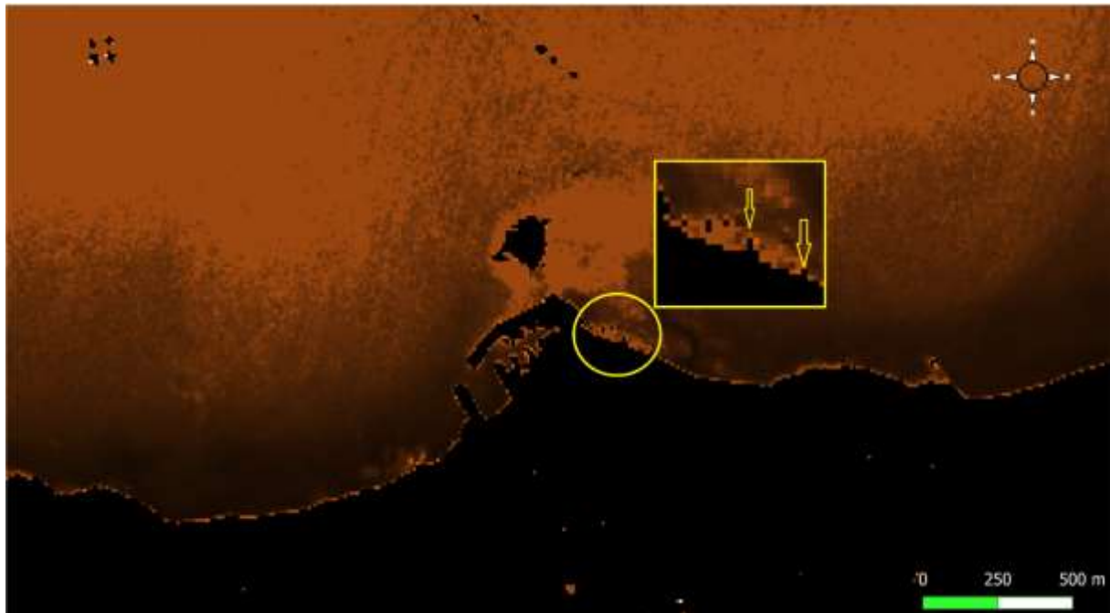
Figure 08. Use of the NDWI (Normalized Difference Water Index) fot the identification of Submerged Structures on the harbour site of Iomnium
