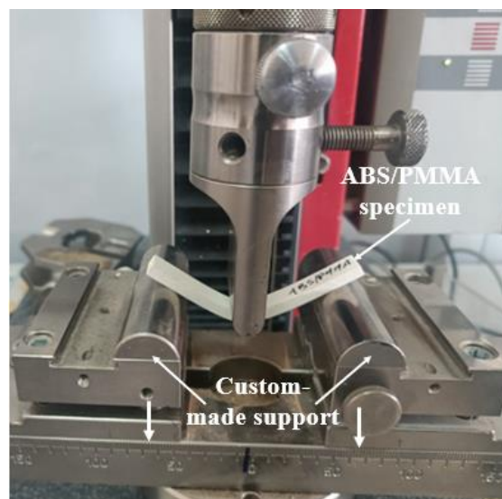
Fig.1. Three-point bending specimen mounted on custom-made supports during test.
