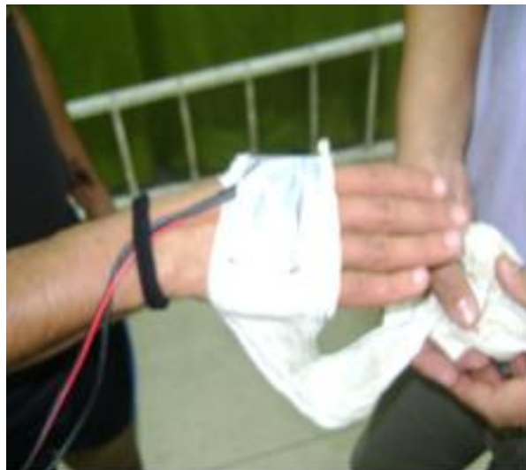
Fig. 2. Accelerometer placed on the operator's hand for stimulation.
