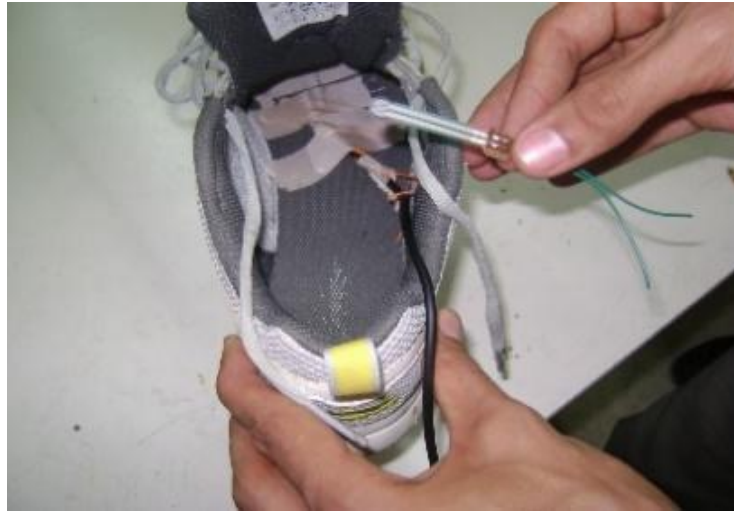
Fig. 3. FSR Sensor and Connection Wiring in an Athlete's Shoe.
