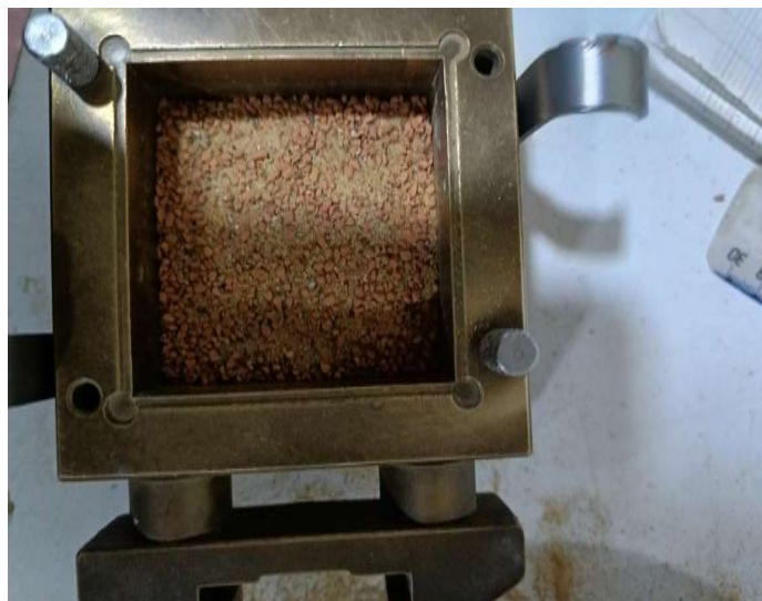
Fig. 11 – Filling the box with the sand-silt mixture + 1mm brick waste.
