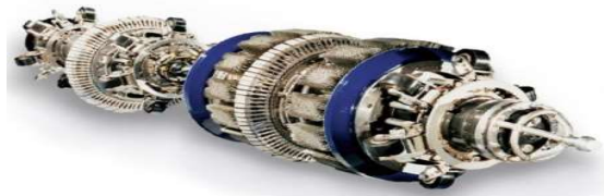
Fig. 4 – The intelligent MagneScan HR tool[24]
