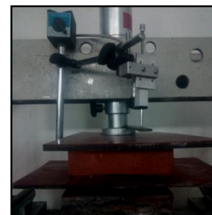
Fig. 3 – Adobe testing machine.
