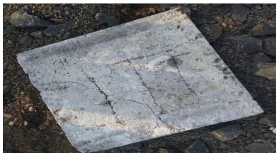
(c) Concrete with 1.5 % fibre content –A2
