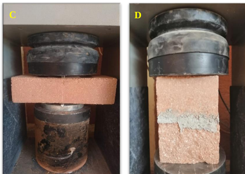
Fig.7 – Dry strength test: C) Dry tensile strength; D) Dry compressive strength.
