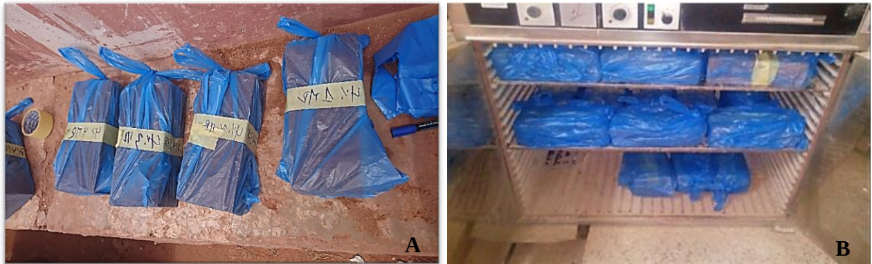
Fig. 6 – Curing conditions: A) Storage in the laboratory, B) Storage in an oven.
