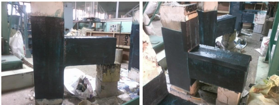
Fig. 7 – Retrofitted beam column joint specimen
