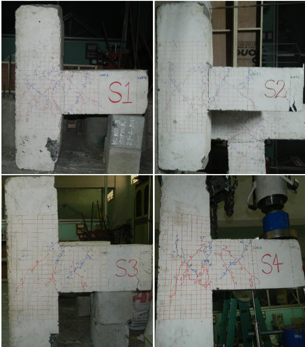
Fig. 4 – Damaged Specimens after testing (S1, S2, S3, S4)
