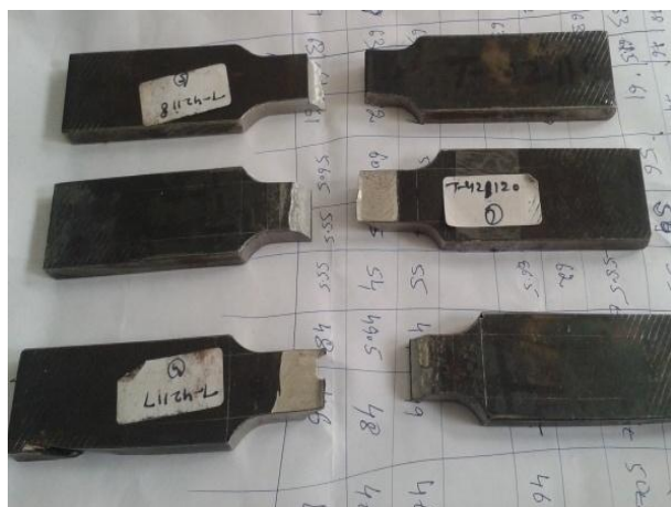
Fig.11- Samples of welded plates after tensile loading
