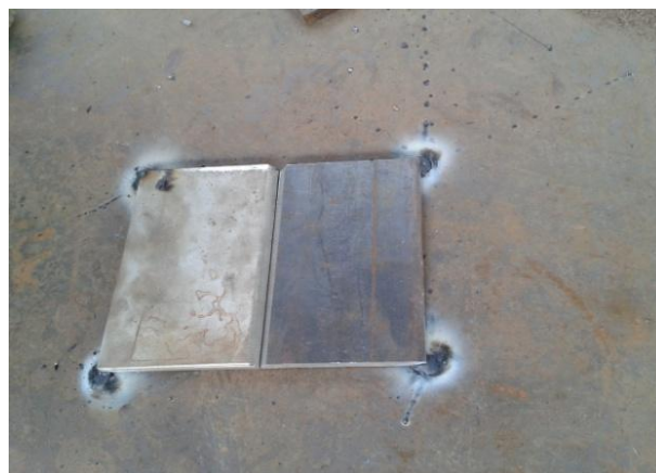
Fig.1 - Plates before Welding Process Having V groove at Center
