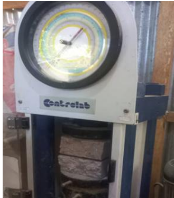
Fig. 4 - The SCEB brick during the crushing test
