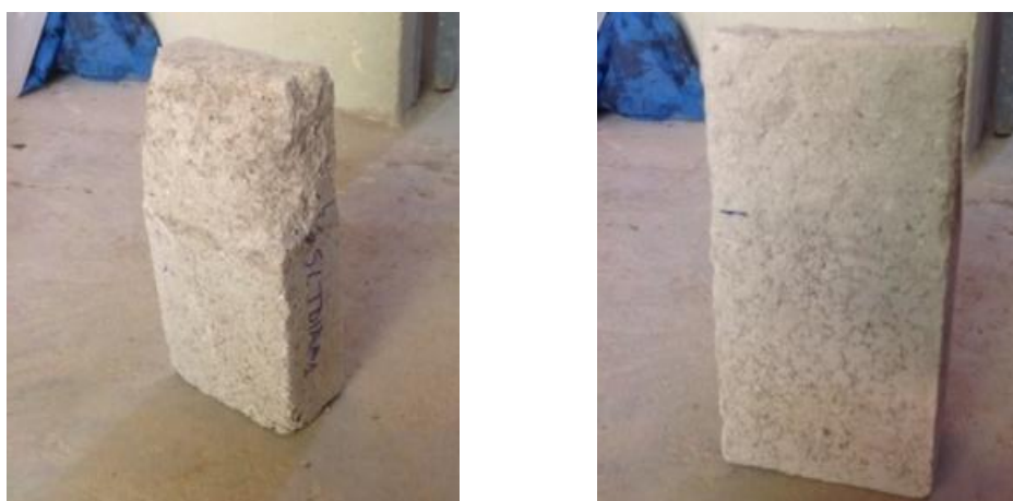
Fig.10 Appearance of SCEBs 100D0C (left) and 94D6C (right) bricks after immersion test
