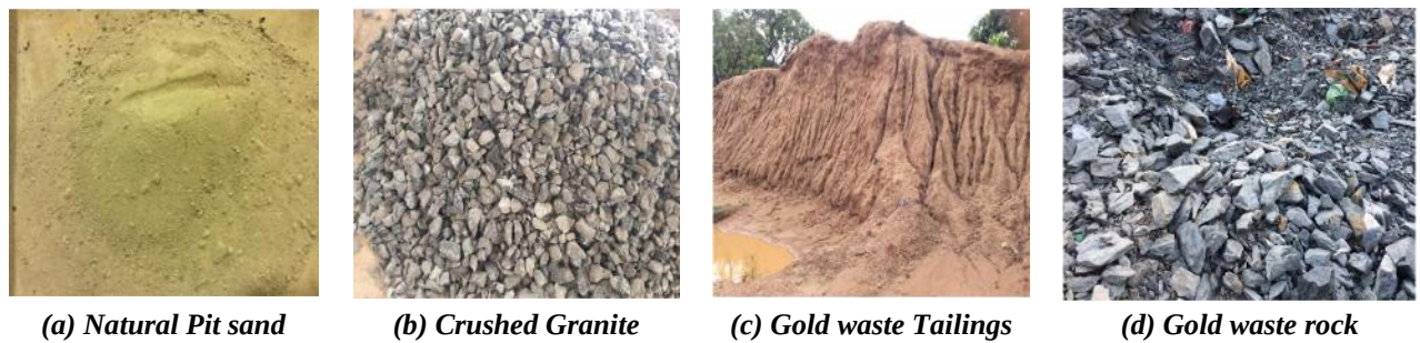
Fig. 1- Sample of pit sand, crushed granite, goldmine tailings and waste rock from the source for the experiment
