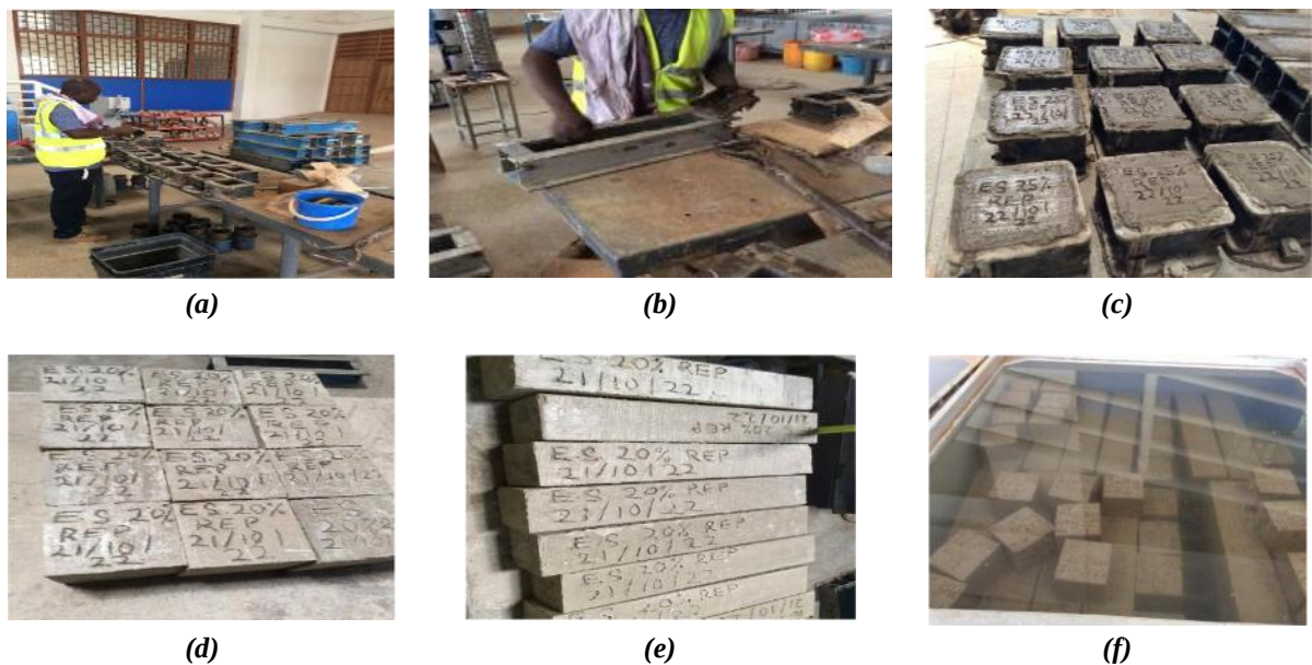
Fig. 4 - (a& b) Oiling of BS moulds 100x100x100 and 100x100x500 (c) specimen concrete inside cube mould, (d) specimen concrete out of cube mould, (e) specimen concrete beams (f) Specimen in a curing tank
