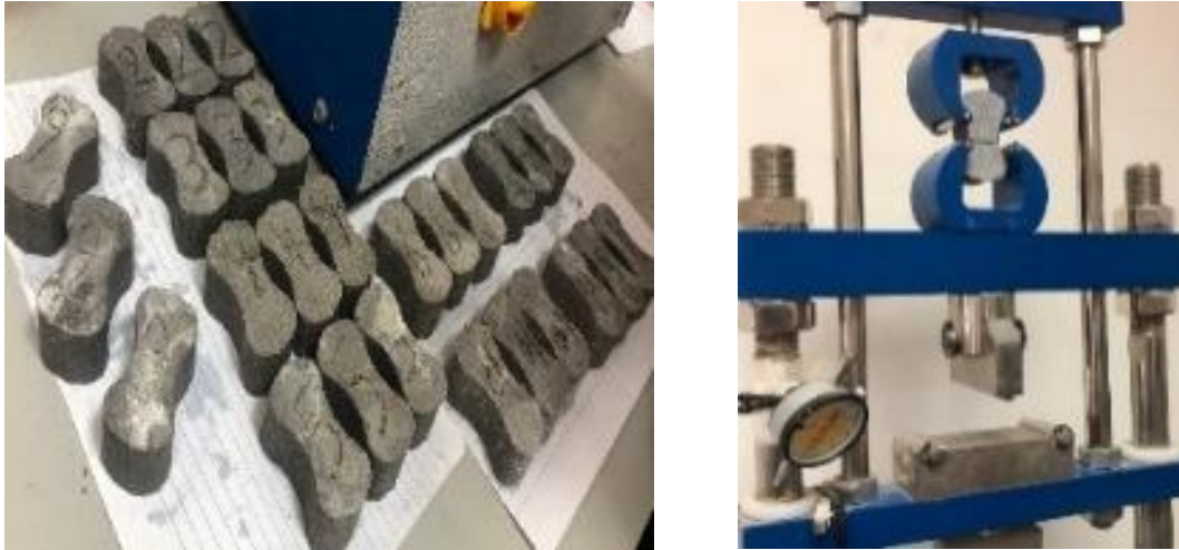
Fig. 7 - Tensile test according to ASTM C307.
