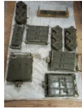
Fig. 4(e)- Pouring mortar into the form and then curing it.
