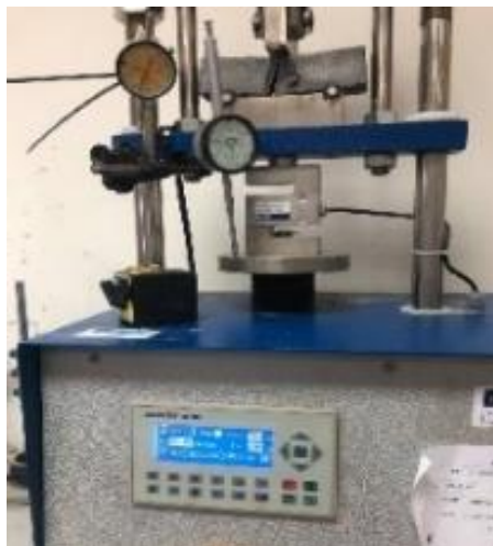
Fig. 8 - Flexural strength test according to ASTM C348.
