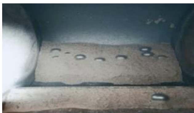
Fig. 2 - The Los Angeles device crushed the bottle glass into fine, small fragments.
