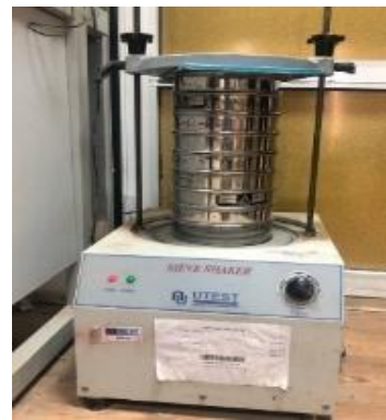
Fig. 3 - Sieve analysis for crushed waste glass.
