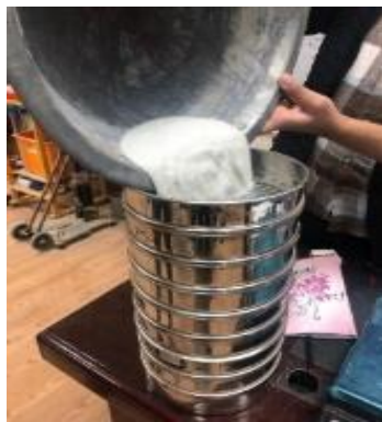
Fig. 3 - Sieve analysis for crushed waste glass.
