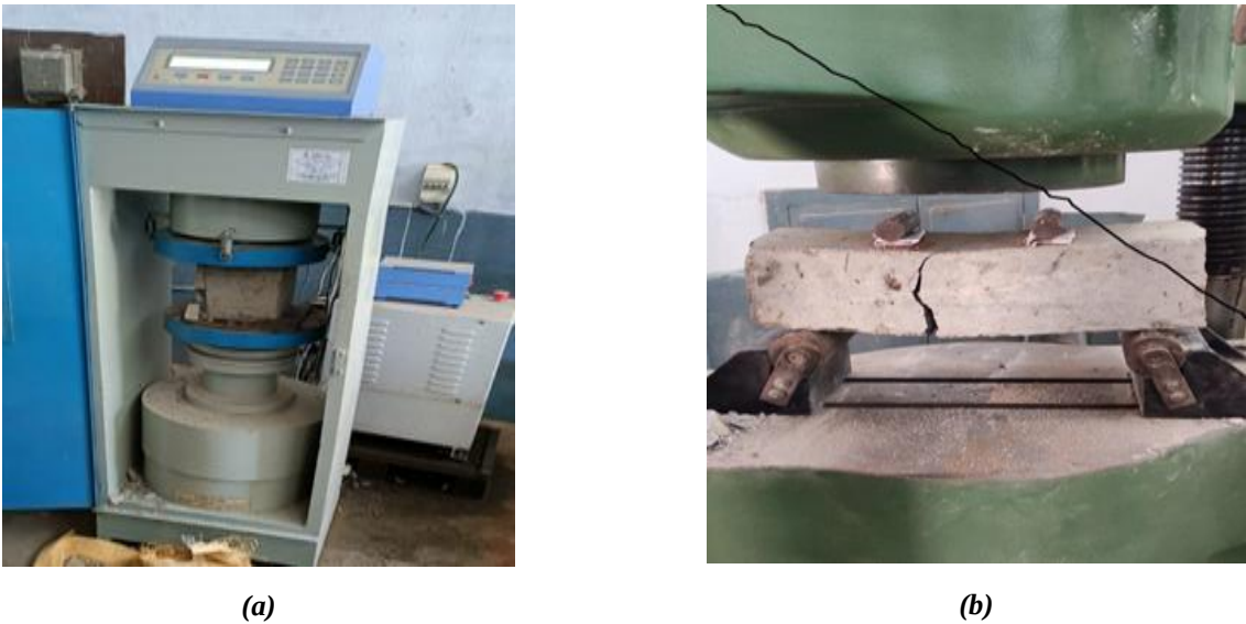
Fig. 1 – (a) Testing of specimen for compression; (b) Testing of specimen for flexure
