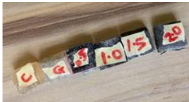
Fig. 4- Specimens for the water absorption
