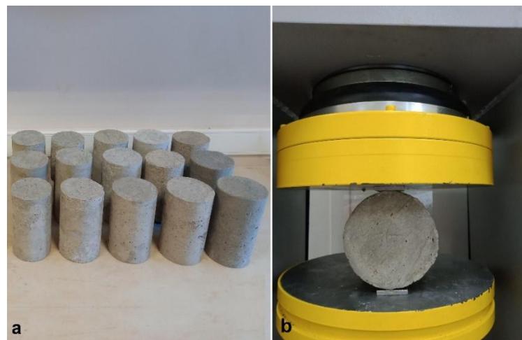
Fig. 4 – a) Brazilian (splitting) tensile strength (BTS) test specimens, b) a photo from the BTS test
