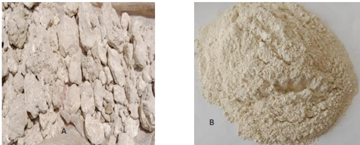
Fig. 1- (A) Drying process of the clay sample, (B) grinded and sieve clay sand
