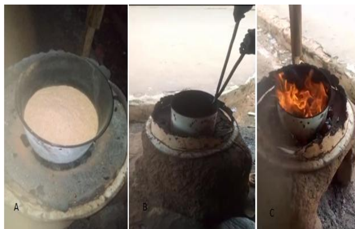
Fig. 2- shows the calcinations process of rice husk ash.
