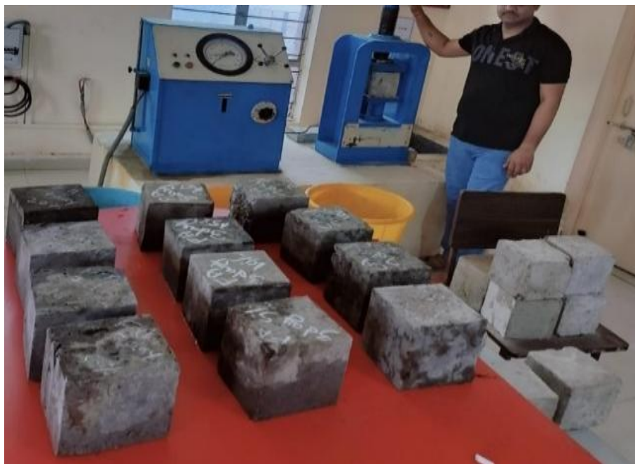
Fig. 8 - Compressive Strength Test Performance
