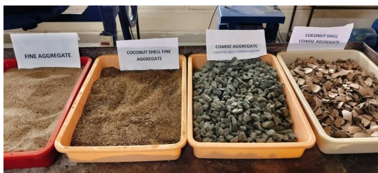
Fig. 5 - Prepared Fine Aggregate, Coconut Shell Fine Aggregate, Coarse Aggregate, and Coconut Shell Coarse Aggregate
