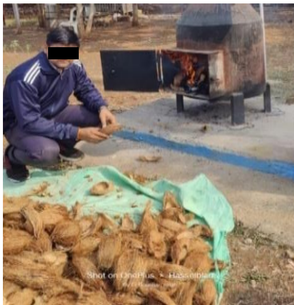
Fig. 4 - Preparation of Coconut Shell Ash
