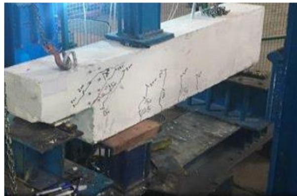
Fig. 6- Dapped end beam under test
