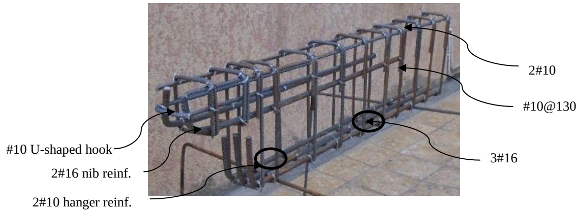
(a) Details of Reinforcement for Control Beam
