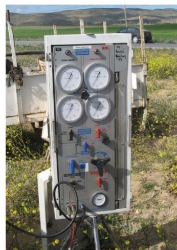
Fig. 1 - (a) Procedure of the Ménard pressuremeter test, (b) Pressuremeter tests in the study site
