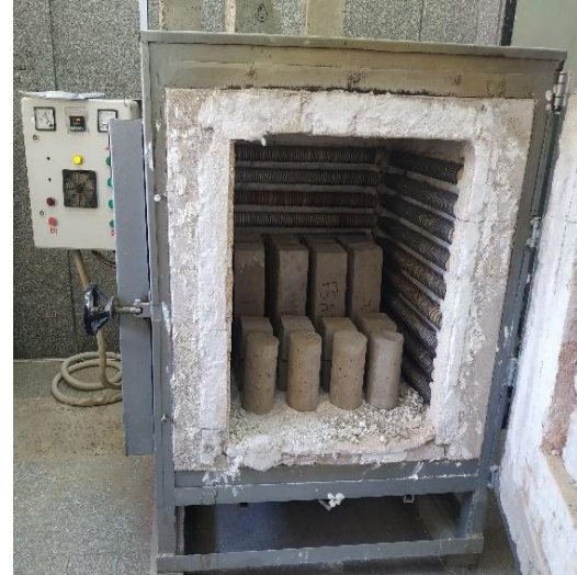
Figure 4 - Concrete specimens inside the furnace
