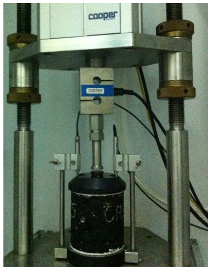
Fig. 2 – Dynamic modulus test on asphalt concrete using Cooper press.
