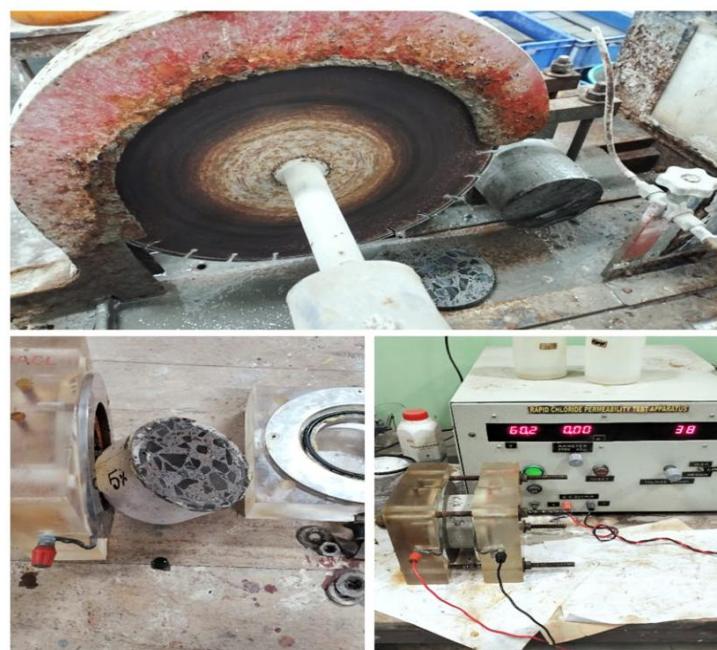
Fig. 17 – RCPT test on cylindrical specimen
