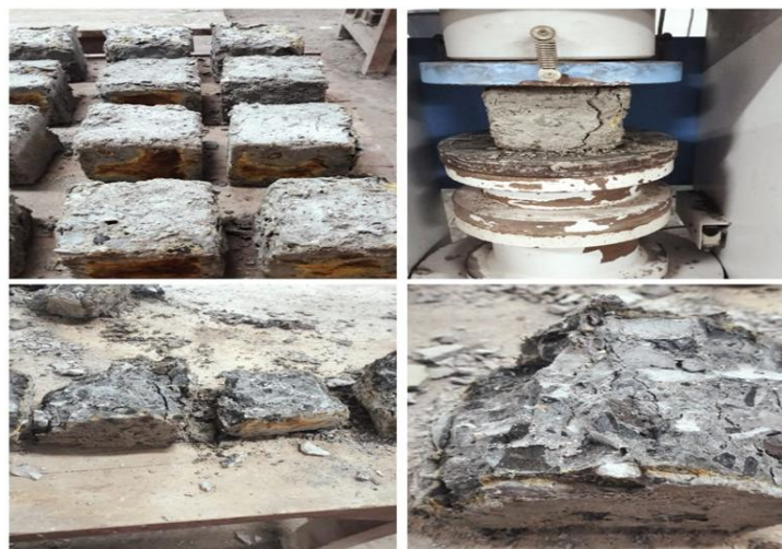
Fig. 15 – Compressive strength test on acid exposed specimen
