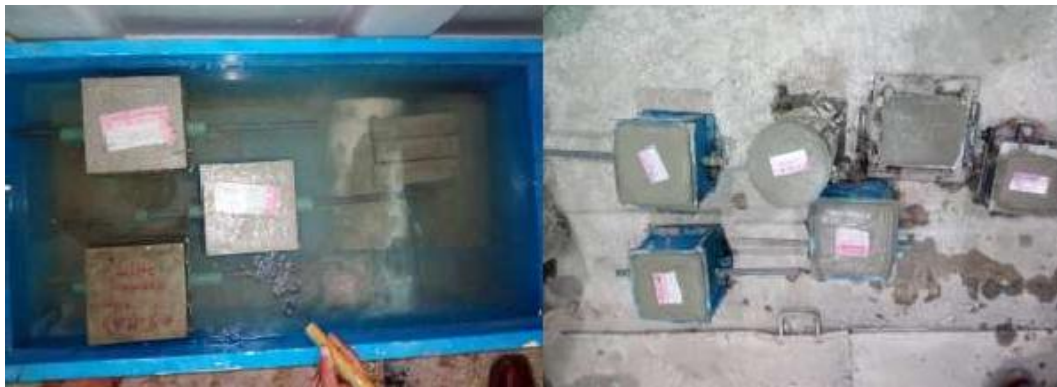
Figure. 4- illustrates the curing and molding process
