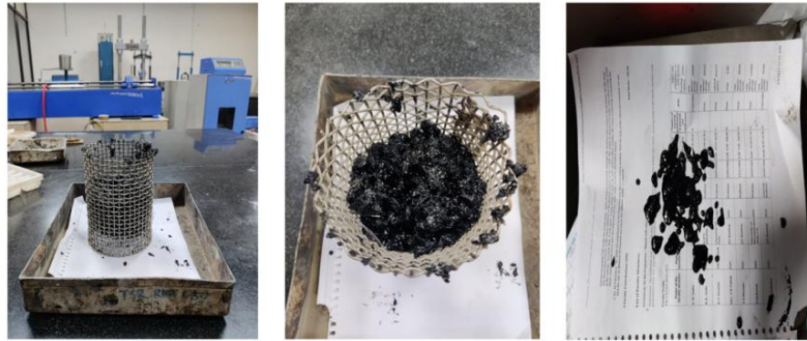
Fig.2 - Drain down testing setup and binder retention.
