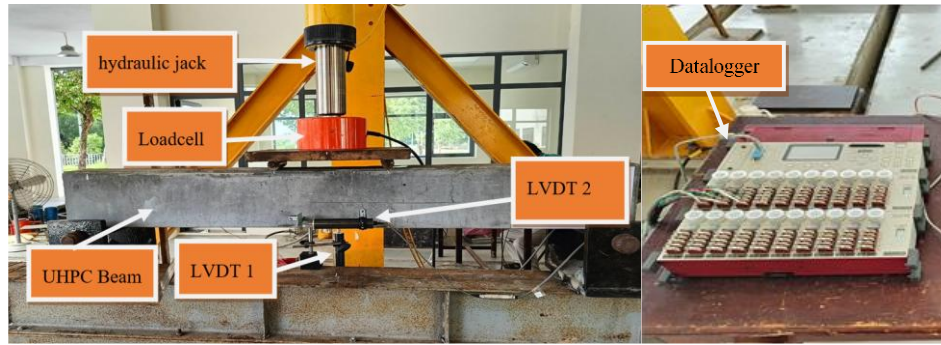
Fig. 7 – Installation of experimental equipment
