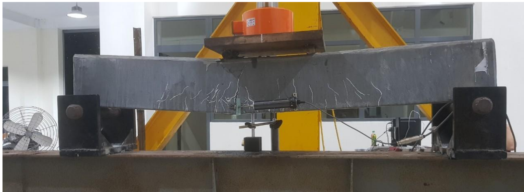
Fig. 10 – Cracking of UHPC beams contain RHA
