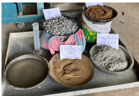
Fig. 2 – Raw materials (cement, FA, superplasticizer, water, fine and coarse aggregates).
