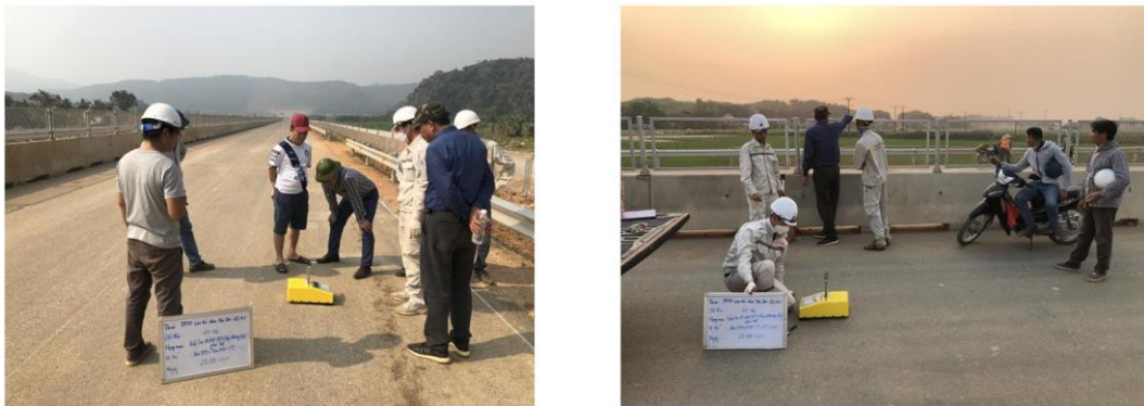
Fig. 3 – Measurement of density by PaveTracker 2701 – B and Coring for calibration
