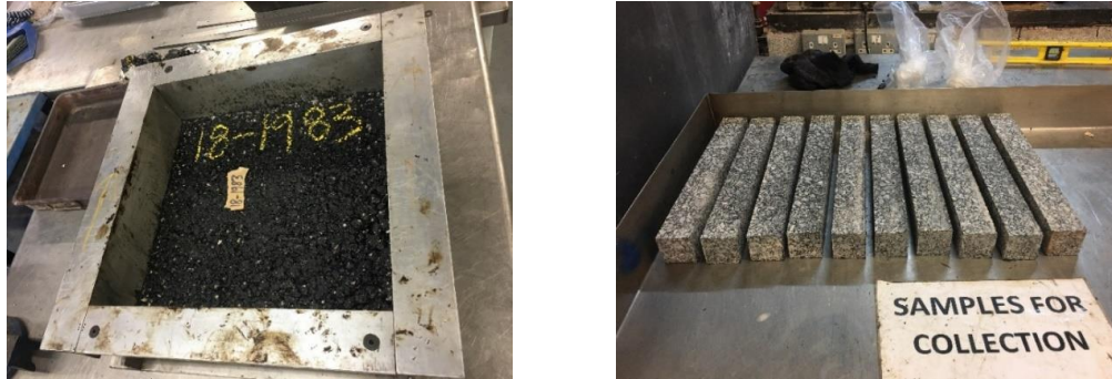
Fig. 3 – Large Slab and Beam Specimens for 4PBT
