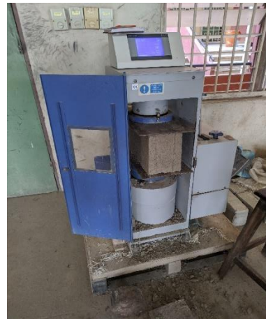
Plate 6- Compressive strength test
