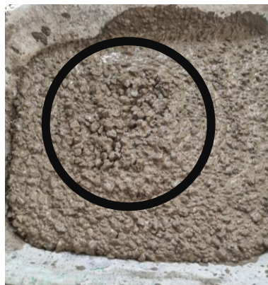
Fig.12 -Segregation occurred in the ACI211 mixture (NW.S + CS)
