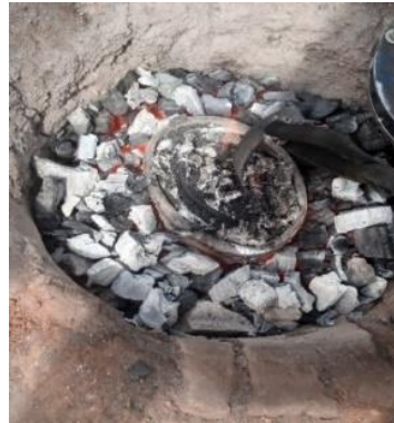
Fig. 12 – Melting of the aluminium scrap in a bail-out furnace
