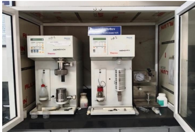
Fig. 2 – Mercury intrusion porosimetry test setup
