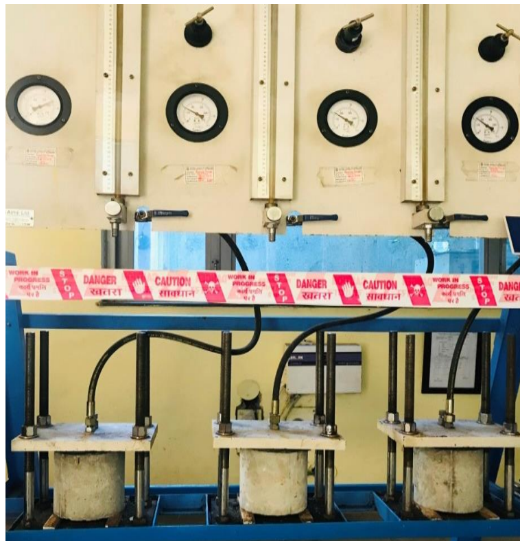
Figure 7- Water permeability test set up
