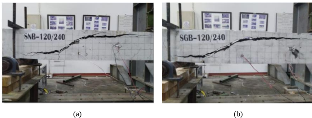
Fig. 12 – Failure crack (a) Normal concrete and (b) Geopolymer concrete [31].
