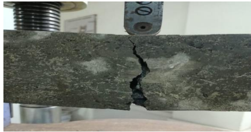
Fig. 13 – Flexural failure of beam with plastic aggregate
