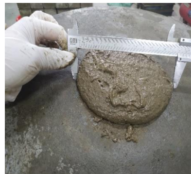
Fig. 3 – Flow test of GP mortars
