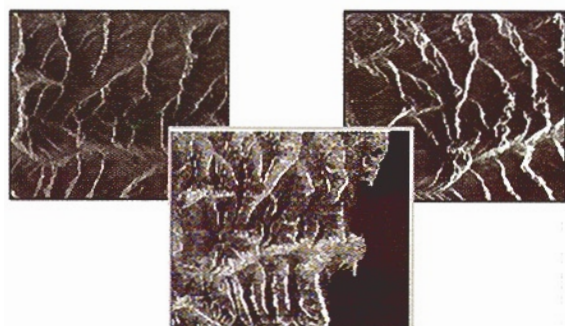
Fig. 2 ADM SAR Ascending/Descending Merge sample product (middle) through combination of ascending (left) and descending orbits (right).
