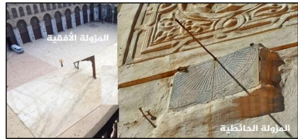
Figure 12: Two sundials made by Ibn al-Shatir in the Umayyad Mosque in Damascus
