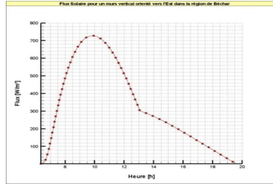
Figure 3. Solar flux to a vertical East wall.
