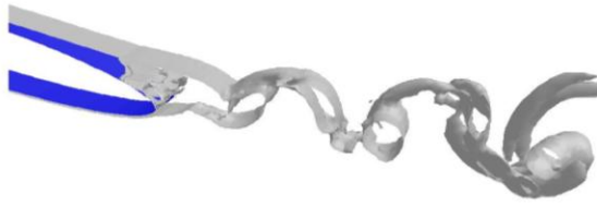
Figure 9. Instantaneous isosurface of the vorticity magnitude for 3D DES ( \alpha = 18.45^\circ )
