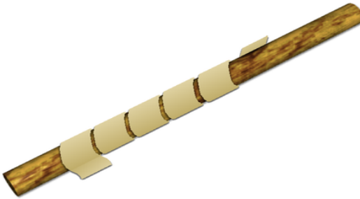
Graph 1-1 A Scytale: An Early Device for Encryption.
